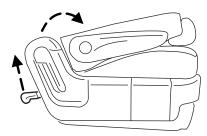
Continuing to lift the handle will tumble the seat forward, allowing easier access to the third row seat.
